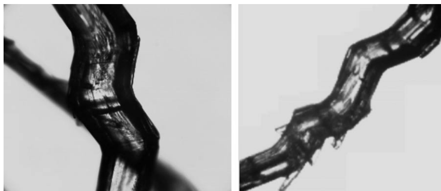
Figure 13. Crystals of 135C246I : 135B246M : triple hinged (w-type) crystal (left) and multiple-hinged ("alkyl-chain" type) crystal (right).
